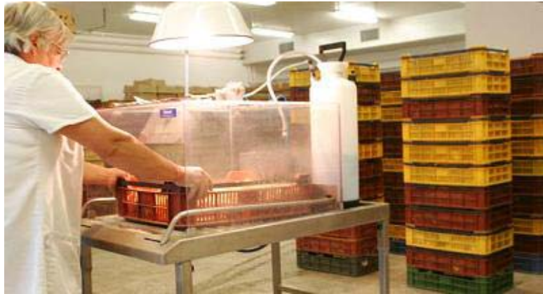
Cabinet sprayer (Desvac Hatch Spray)
